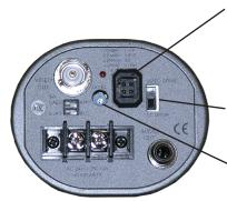
AUTO-IRIS CONTROL CONNECTOR MANUAL SWITCH FOR SELECTING BACK LIGHT COMPENSATION OR TURNING OFF COMPENSATION ENTIRELY. USEFUL IN CERTAIN LIGHT/ ENVIRONMENTAL CONDI-TIONS
